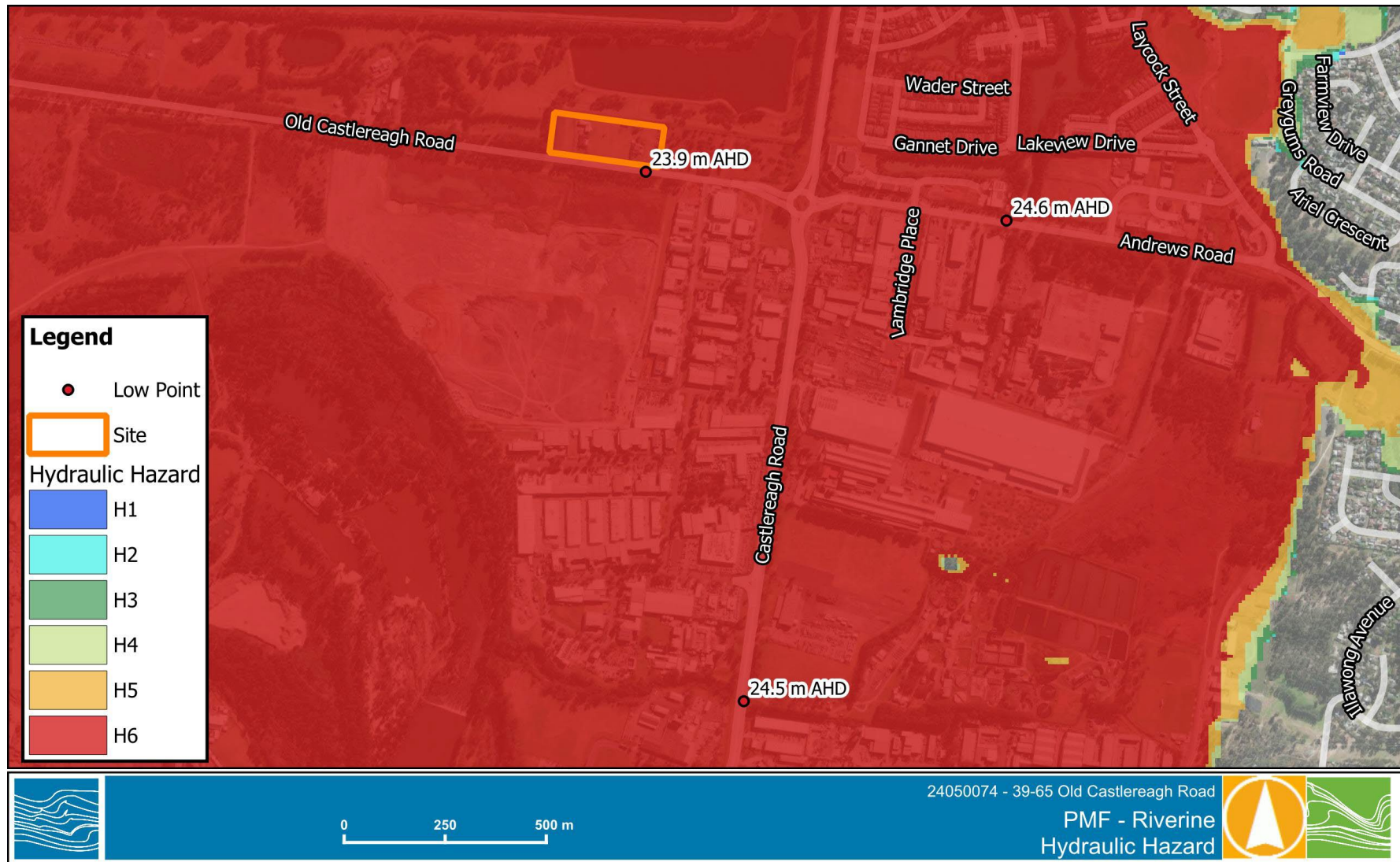
Figure 12 Hydraulic hazard in the riverine PMF
